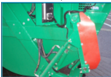
Externally mounted hydraulic hose
