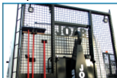
Impact tested head board
